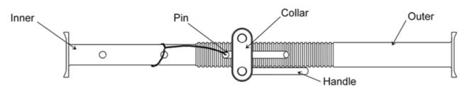
The strut end plates have turned claw like corners designed to "bite" into timber.
